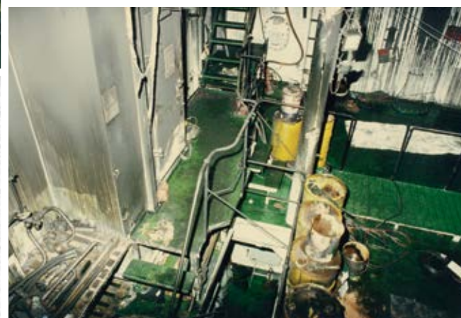
TOP: After the fire aboard the British Adventure, much of the items in the steering gear room (where the fire occurred) was covered in soot.
