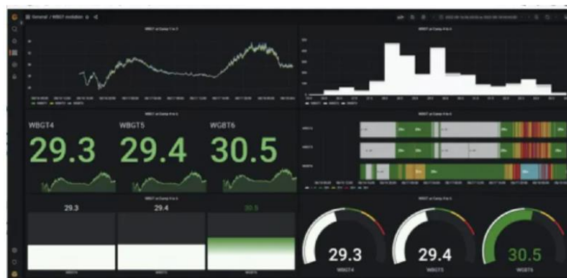
Figure 4: Real-time WBGT monitoring dashboard with alert system
